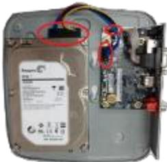
④ Connect the Data cable and power cable to the HDD and the mainboard respectively.
