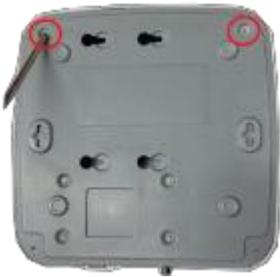
① Loosen the screws on the bottom of the chassis.
