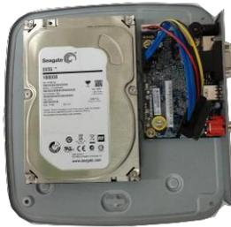
② Align the HDD with the four holes in the bottom.
