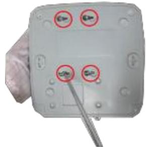
③ Turn the device upside down and then secure the screws (supplied) firmly.
